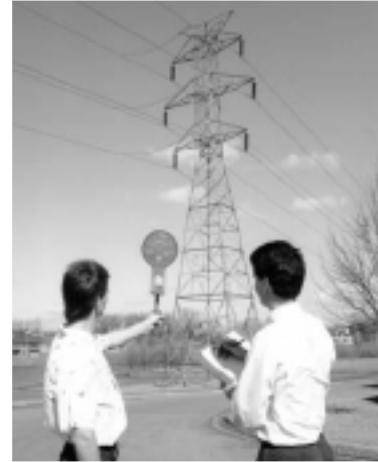
Power Line Survey Instrument Wide Dynamic Range On-Board Data Logging Combination E & H Readings
